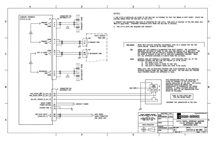
The example Application Note [above] is for the U1713-2-40 Approach Adapter. The Application Note identifies the ports used and how they are wired to other systems. The STC developer uses the Application Note [and this Installation Manual] to develop detailed Installation Drawings and to help develop Ground Test Plans and Flight Test Plans. Canaan Avionics uses the Application Note to communicate and validate the software functionality.
